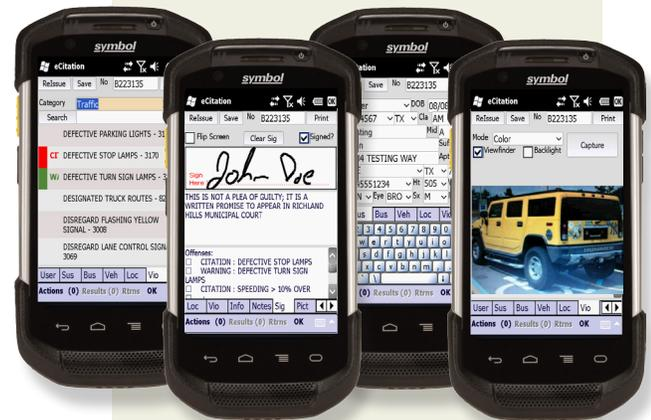
*Brazos handheld devices interface with state DMV lists to eliminate data entry errors on citations.*
